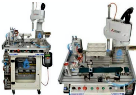
SCARA Robotic Cell
