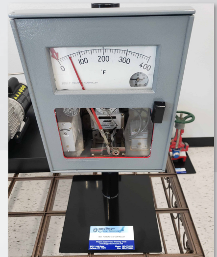
Foxboro 43 AP Controller Cutaway (128-FAPC)
