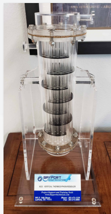
Vertical Thermosyphon Reboiler Model (115-VTR)
