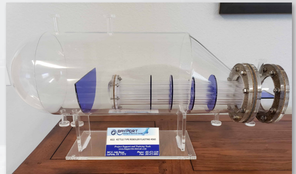
Kettle Type Reboiler Floating Head Model (115-KRFH)
