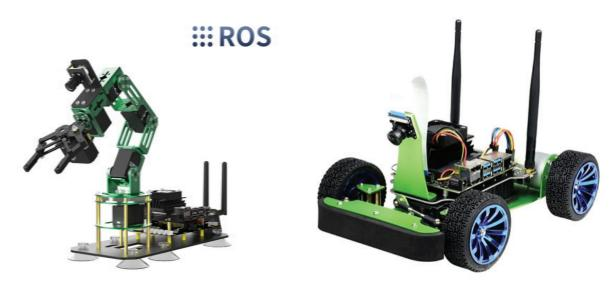
This hardware setup includes Robotic Arm and Car which can used to implement AI skills using Embedded GPU Kit & Robotic Operating System (ROS) by building applications.
