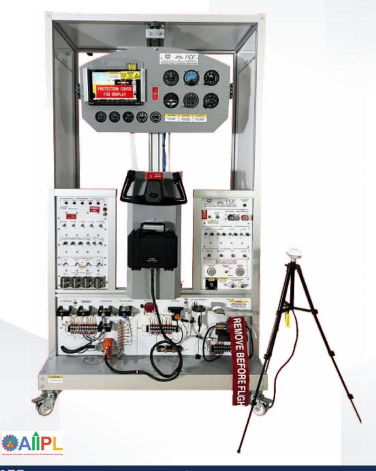
Aircraft Cockpit Instrument Training Set(CBT-100B) is a complete and fully functional simulation of typical aircraft cockpit. It includes essential flight, engine and pitot-static instruments. This training set provides hands-on maintenance training while also functioning as a demonstration tool for instructors. It demonstrates the principles of gyros, altimeter and the engine instruments, and also can be used for teaching of instrument removal and replacement.
