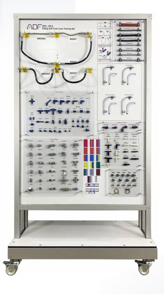
The Fluid Lines & Fittings Trainer Set demonstrates multiple types of fluid lines fittings and their assembly techniques. It displays the aircraft standard for assembling, routing, supporting fluid lines. Examples of frequently made mistakes are shown as well for trainees to avoid.
