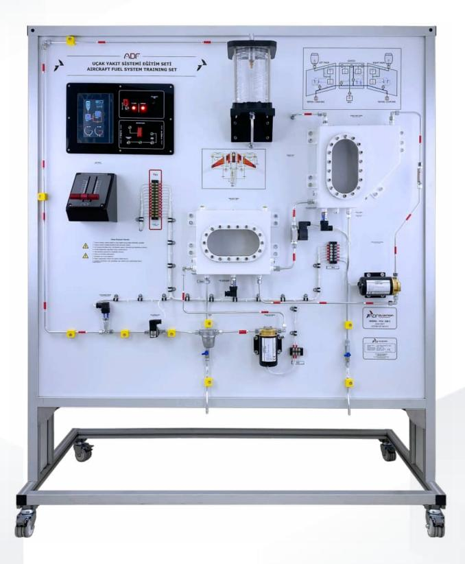
Designed to represent a complete aircraft fuel system, Model FCU – 100B Turbine Fuel System Training Set enables trainees to learn the essentials of fuel system components and how these components are linked to each other in a typical aircraft fuel system. This trainer includes a capacitance fuel system that shows non-linear fuel quantity indications. It comes fully plumbed and with a wing tank.
